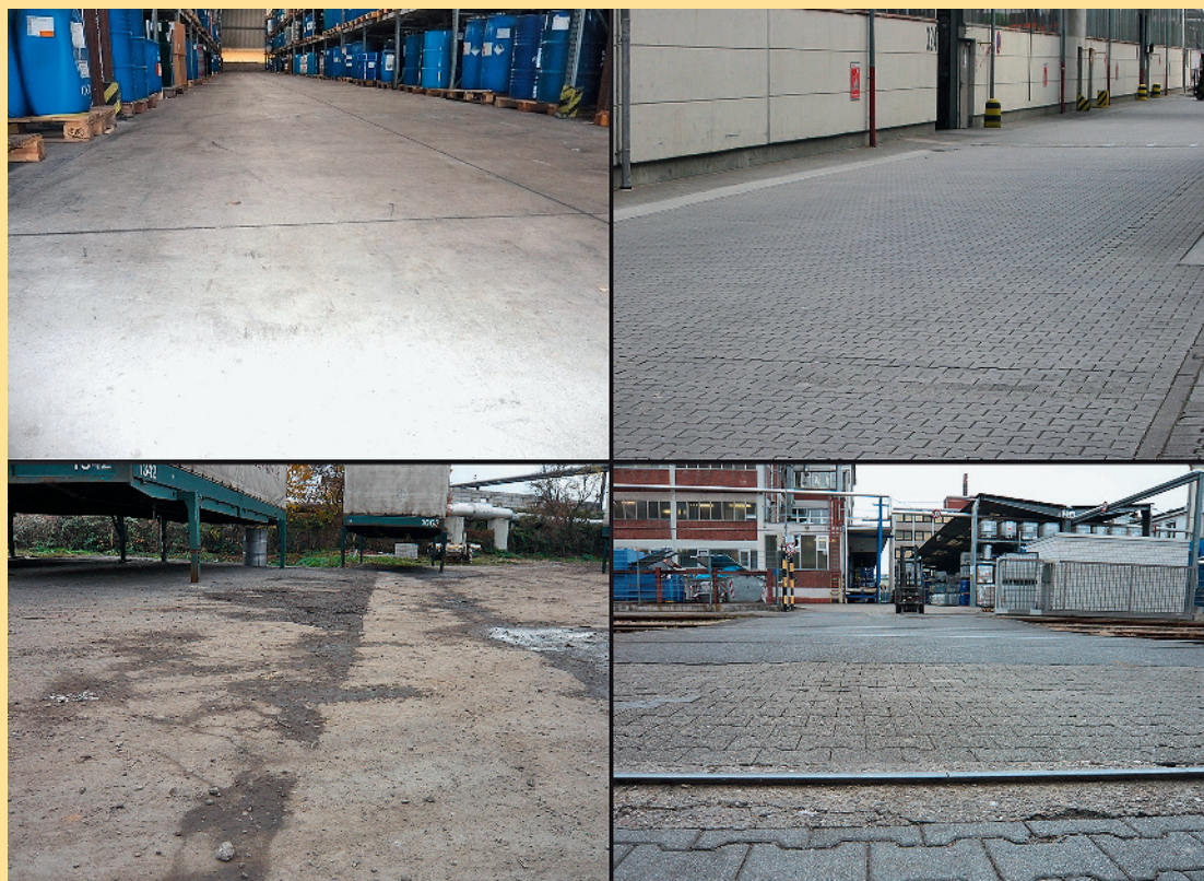
Figure 1: Four test tracks of the series of measurements 1: planar concrete in a roofed open-air storage (top left), concrete composite plaster outdoor (top right), concreted open air ground with holes and cavities (bottom left) and level-crossing with train rails and rails of gates (bottom right).
